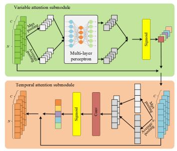
Figure 2. The architecture of the proposed 1D-DAM.
