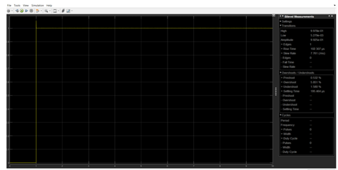
Figure 10. LQT step response display without noise.
